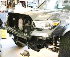
9.) This is how the bumper will look with the lower section cut off. Not shown in this picture are the inner fender liners which will also need to be trimmed. Trimming the inner
