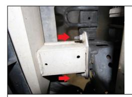
12.) The crash bar has 6 bolts total 3 per side holding it on. You can now remove those and discard the crash bar. There are two nuts on the out side and one on the inside. (different crash bar shown but same method applies. In our video of the FJC bumper install on <a href="https://www.youtube.com/watch?v=dF-B7inrDyU">https://www.youtube.com/watch?v=dF-B7inrDyU</a> you can see this action done as well. 2min 55 sec into it.
