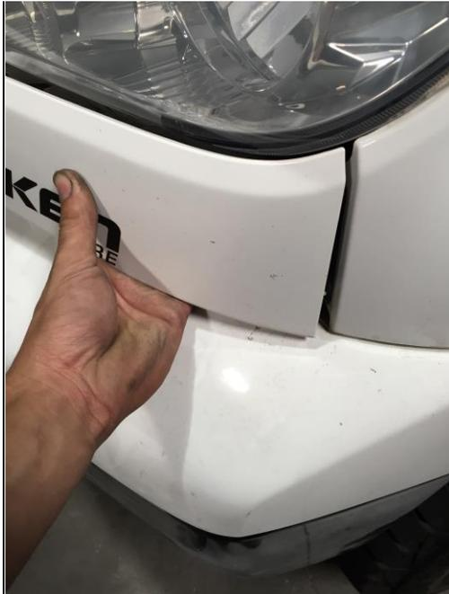
Step 3.) Now that the plastic clips are removed you can gently pull on the light valance piece "straight out". NOTE Pulling it sideways may result in broken fasteners.
