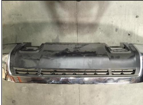
Step 12.) Double check that all hardware and plastic clips are removed, remember some models may have more or less of each. Also be sure to check your wire connection for fog lamps and or parking sensors are free and clear of the bumper. Once you are sure the bumper is free you can now remove the stock bumper.
