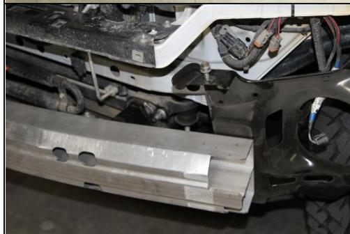
13.) you are now ready to remove the aluminum bash bar found behind the stock bumper. This bash bar is held on with 3 nuts per side 6 total nuts. Remove all the nuts and remove the bash bar. A 17mm socket with a short extension and 3/8in ratchet is ideal.
