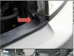
**OPTIONAL:** On 2003-2005 models have a small plastic piece that attaches to the factor bumper. This can be unclipped from the factory bumper and lined up below the grill. It will require drilling two small 1/4in holes in the factory head light mount and re-using some of the factory 10mm screws. This is optional and not required.
