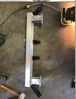
6.) There should be 4 factory studs sticking out from the frame on both sides. The outer three on each side will need to be removed. Use a mini sledge or large hammer to hit them at a 45\* angle. If you hit them right, they will pop right out. Leave the two inner studs in place to help align the bumper on the 4runner.
