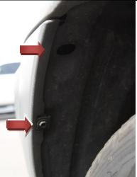
2.) on the out side edge of the stock bumper you will find 12 10mm bolts and screws. They are located in each fender well, under the bumper and under the grill. Remove all these bolts and screws. Different models and years may very in the quantity of bolts and screws. So take your time and remove all the hardware that holds on your factory bumper.
