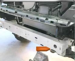
5.) Once the factory bumper is removed you will find a metal bash bar that is held on to two boxed brackets. You will need to use a 14mm deep socket and extension to remove the bash bar. Then use the same socket to remove the brackets on both sides of the frame.
