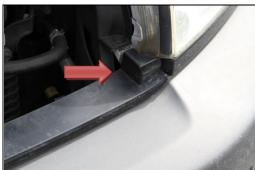
**OPTIONAL:** On 2003-2005 models have a small plastic piece that attaches to the factor bumper. This can be unclipped from the factory bumper and lined up below the grill. It will require drilling two small 1/8in holes in the factory head light mount and re-using some of the factory 10mm screws. This is optional and not required.
