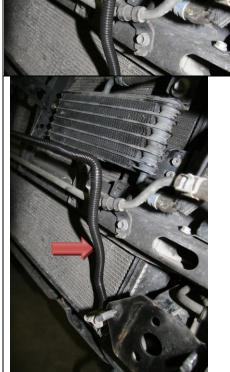
8.) Carefully bend the AC line near the bottom where the bumper would make contact. This should be done very carefully and be sure to check clearance again once you mount the bumper. We also provide a protective plastic wire loom for you AC line.
