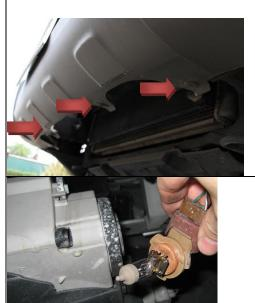
3.) Carefully detach the bumper from each inner fender plastic by gently tugging at the bumper, working your way up and down and alternating from passenger side to driver side.
