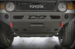
12.)Once the brackets are installed you can now level off the bumper and tighten the brackets. A floor jack is helpful for this or a good friend to hold the bumper in place while you tighten it down.
