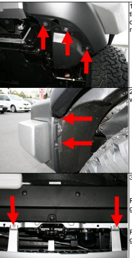
1.) Remove <u>ALL</u> of the factory screws along the bottom of the front bumper corners. Different models may have more or less screw/bolts than shown. Refer to factory screw/bolt removal if it does not match what is shown here.
