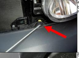
4.) Remove all of the snap rivets along the top of the bumper by gently prying upwards on the center button with a flat head screw driver.
