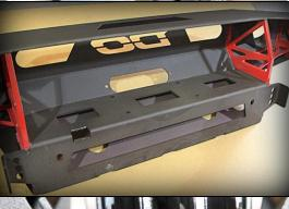
10.) Install winch controls. There are many different styles of winches and controllers to make a one size fits all. But there is a significant amount of space inside the bumper to mount a control box in several different locations. Find the best location that fits your needs the best.
