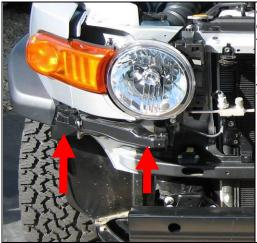
8.) Remove the factory side bumper supports and the front cross bar that span the distance across the front between the side supports.
