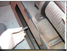
9.) Install winch. Place your winch on the mounting plate on the back of the bumper. Using the mounting hardware that was supplied with your winch, bolt the winch to the mounting plate. Please ensure that your winch mounting hardware is tightened according to the manufacturer's specifications.
