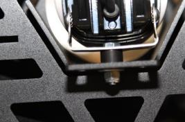
Note: if installing lights this is the time to do it. Some lights will require a spacer like the baja designs do, shown in picture. Check to make sure light is centered in the hole before going further.
