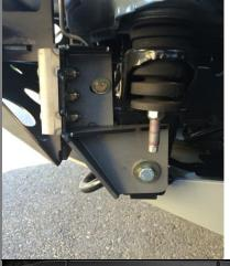
11.)Once the bumper is slid on the bumper installed you can now use the supplied reinforcement brackets to clamp and secure the bumper to the frame. The supplied M12 metric bolts thread into the bottom portion of the bracket and the supplied M8 threads into the upper portion of the bracket. You will also run the 3/8in bolts through the bracket, bumper and frame as shown above.
