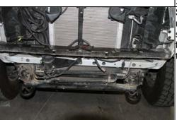
Step 15.) Now that the bash bar and frame horns are removed you have an exposed set of frame rails. Your next step will include a hammer and careful inspection of the frame and all exposed parts. This is also a good time to touch up a rusty frame with spray paint or under coating.
