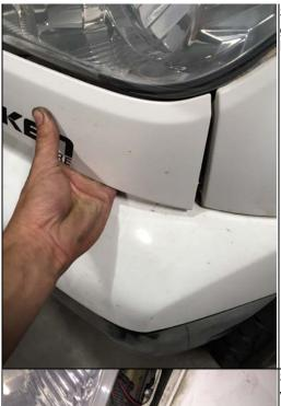
Step 3.) Now that the plastic clips are removed you can gently pull on the light valance piece "straight out". NOTE Pulling it sideways may result in broken fasteners.
