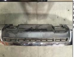
Step 12.) Double check that all hardware and plastic clips are removed, remember some models may have more or less of each. Also be sure to check your wire connection for fog lamps and or parking sensors are free and clear of the bumper. Once you are sure the bumper is free you can now remove the stock bumper.
