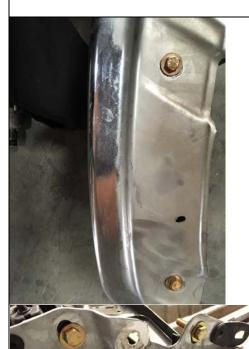
Step 8.) Once all the bolts and clips are removed, you should now be able to remove the top piece. Note some vehicles may have extra clips or bolts. Be sure to check to make sure they are all removed before pulling on top piece.
