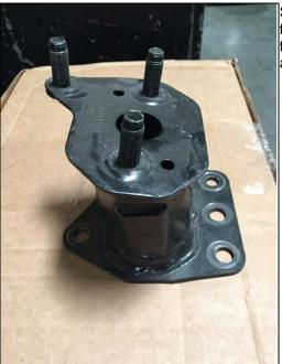
Step 14.) you will also need to remove the steel frame horn from the frame. It has 4 bolts for each one with a total of 8 for both sides. The bolts are 14mm as well and you can use a socket and racket or box end wrench.
