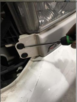
Step 2.) Remove the two black clips on either side on the fill piece under the head lights. Carefully use a small flat head screw driver to pop the rivets out. (DO NOT DISGUARD) You will re-use these clips.
