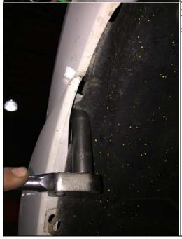
Step 5.) Remove the bolt in the inner fender wheel well. This is a 10mm bolt and can be removed with a racket and socket.
