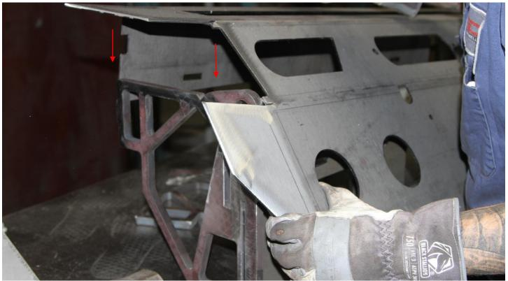
Step 5.) Once you have tacked the two Nevada plates to the winch plate flip it over, so the shackles face you. Then take the "main section" piece and carefully fit it over the witch plate. Also make sure that you have ground the edges of this plate as well shown in the picture above. The main section is a tight fit and has two notches on top of the Nevada plates that it will fit into. Take your time and make sure you center it tight onto the winch plate.
