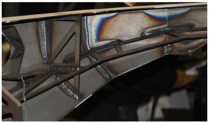
Step 16.) with the bumper removed you can now add the reinforcement pieces to the inside of the bumper. Same rules apply as with other pieces, make sure you dry fit them all first, some grinding/sanding may be necessary for proper fitment. Repeat steps for both sides of the bumper. Be sure to tack them in place on both sides before fully welding the bumper.
