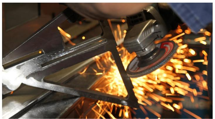
Step 2.) You will need to grind off the scale on the two "Nevada plates" or uprights. Note in the picture where to grind. You can also fit it and see wherever you will weld will need ground for good penetration.
