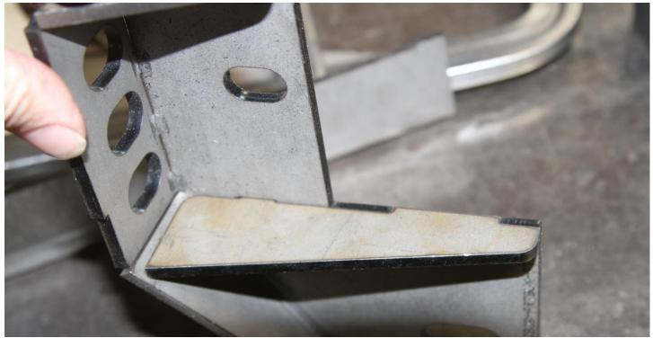
Step 21.) The last and final step is to assemble and weld the reinforcement brackets as shown here.
