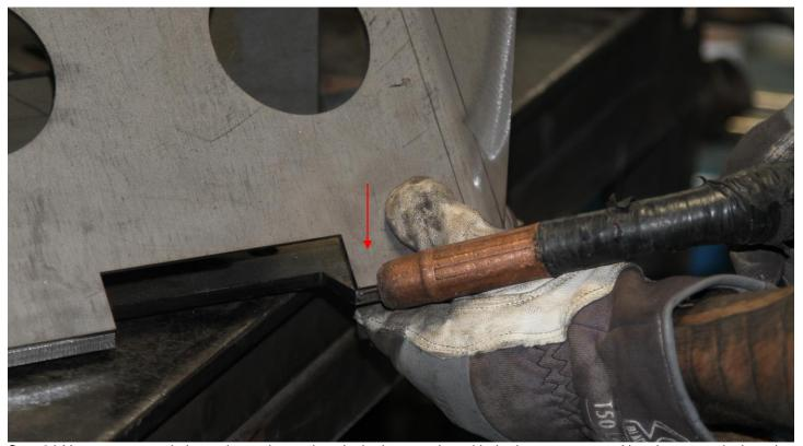
Step 6.) You can now tack the main section to the winch plate starting with the bottom corners. Note how you pinch and hold together the bottom edge of the bumper so those two pieces meet up.
