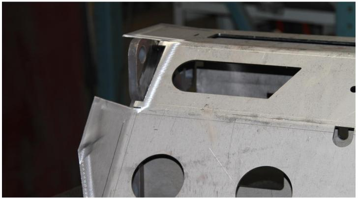
Still Step 5.) note that the shackle when fitted correctly will poke through the front of the skin and fit up flush to main section.
