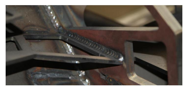
Make sure all the connecting points are fully welded for the strongest bumper possible.
