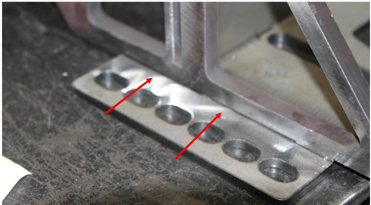
Still step 3.) You will notice that the Nevada plate fits completely flat on the base of the winch plate. Remember the closer the tolerances are the tighter and cleaner the overall bumper will be. Repeat the same steps for the opposite side till both pieces fit snug on the winch plate.
