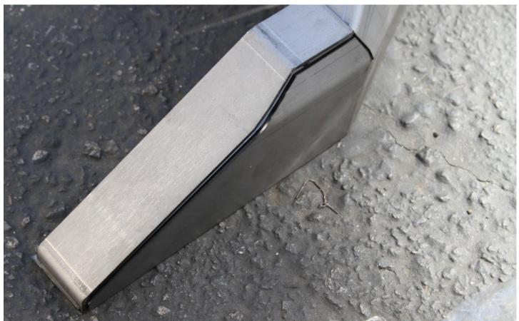
Step 14 tack the D/S filler on both sides as shown. This can be done on the vehicle. Sorry not shown on vehicle.
