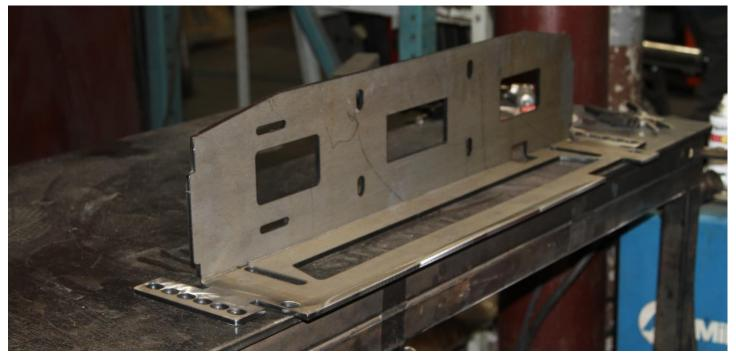
Step 1.) place the winch plate on a flat work bench or welding table. As shown above with the winch mounting surface vertical and the mounting surface flat on the table. The first thing you will want to do with all the pieces is lightly grind (with flapper wheel) all the edges and surfaces that will be welded. As you fit the pieces together this will become apparent to you. Some pieces will need ground down more than others to properly fit. It's best to do a little and test fit.
