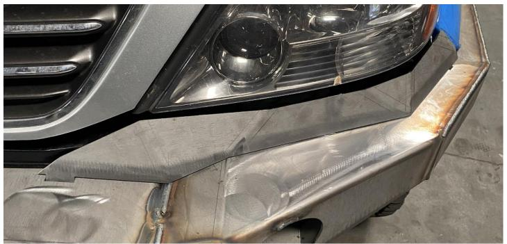
Step 15.) It's time to add the filler headlight piece on each side. Note that some GX sit lower on the driver side causing contact with the filler piece. We recommend 1/4in-1/2in gap along the filler piece between the headlight and bumper. You can use a soft wheel grinder to take down some material. Repeat step 15 on the passenger side as well.
