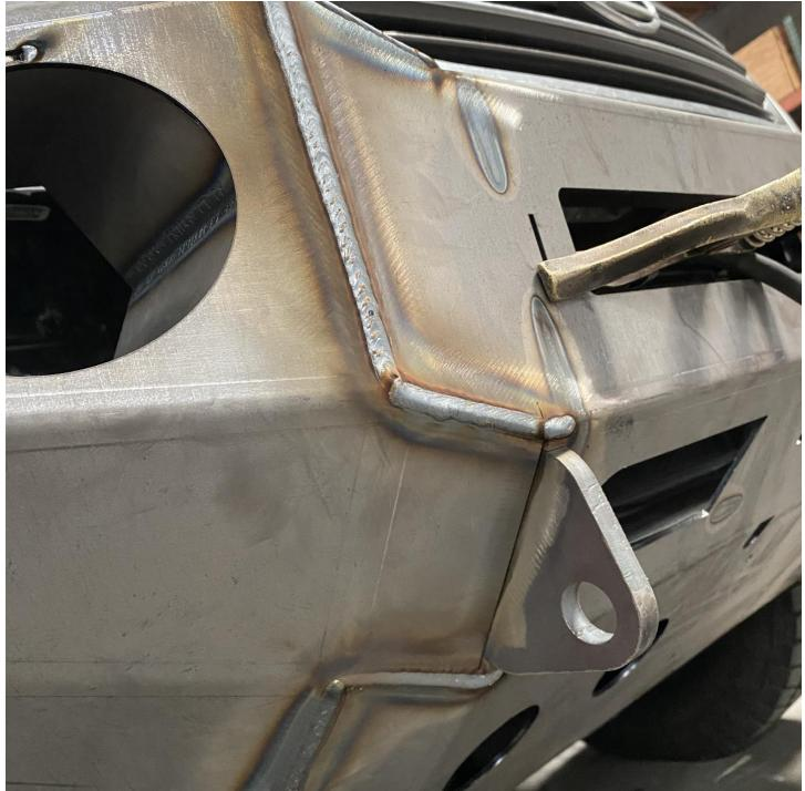
Notice the heated-up areas around the weld and we generally leave the shackle weld for last so that we can do a nice clean weld as that's the only weld you won't grind down and we like it clean ©
