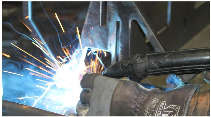
Step 4.) At this point you can "tack" the Nevada plates to the winch plate. We recommend only tacking at this point and doing it in a place that you can easily grind off if you have to go back and change it.
