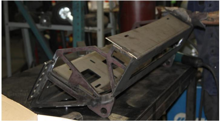
Step.7) Flip the bumper over again so that the top faces you and fit the top piece down into the notches and again tack it into place.
