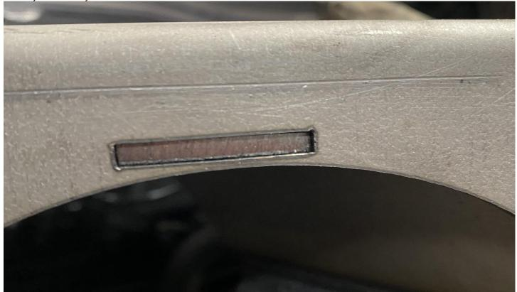
Step 18.) Fit the light holes from the back of the bumper and make sure the tab sits flush into the bumper. You can remove a little bit of material from this part as well to allow good weld penetration.
